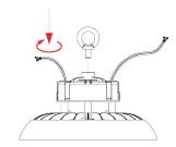
2.Tighten the screw. (This step can be omitted if there is no screw hole.)
