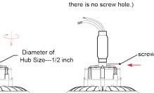
2. Tighten the screw. (This step can be omitted if there is no screw hole.)
